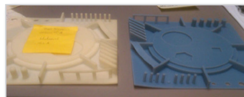
The features in these test patterns appear to be high quality due to a nice surface finish, crisp edges and fine detail, yet they exhibit warping, showing an inability to hold the desired tolerance.
