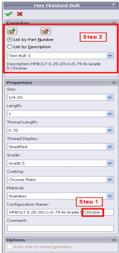
If you open the part file you can see the configurations that have been generated as well as each Configurations Specific Properties.
