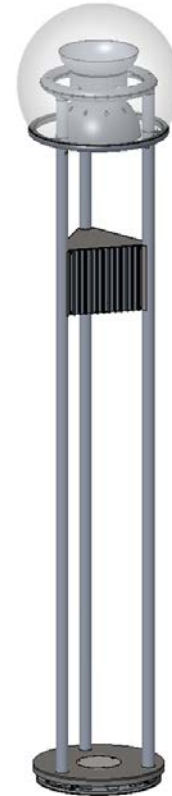
SOLIDWORKS model of the 16 th Street Mall lighting
