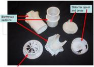
Fan inlet prototype
