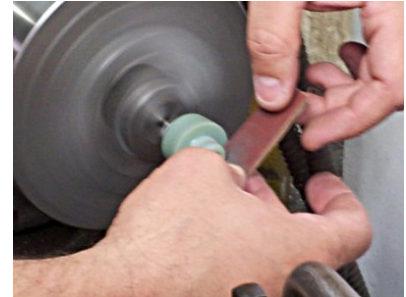
Figure 11: Finishing process of mold component.
