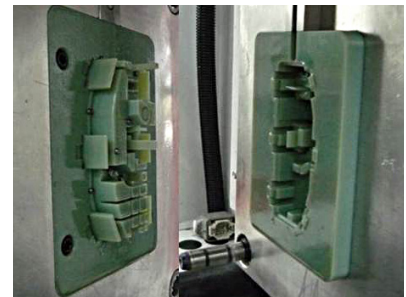
Figure 13: Mold inserts are assembled on a standard steel base and held in place with machine screws.
