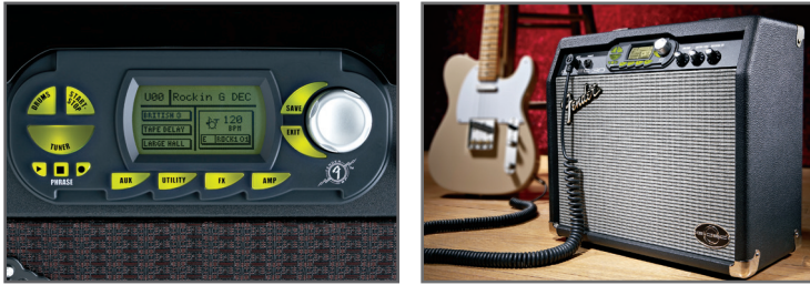
Fender's guitar amplifier prototype printed on an Objet 3D Printer.
