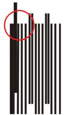
**Target** - The first open gap is visible between the first and second calibration toolpath.
