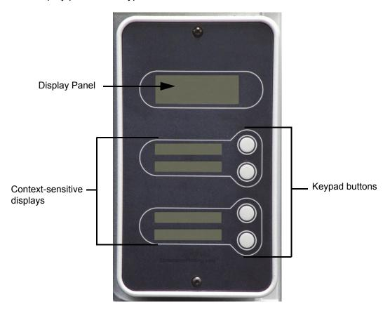
The display panel and keypad are very easy to use, consisting of a larger multiple-line LCD display on top, and four single-line context-sensitive displays, each with one button (or key) below. The top line in the large display always shows system status. The lower three lines of the large display show details related to the current operation.
