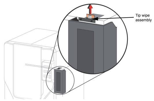
4. Place the new tip wipe assembly over the two mounting posts making sure the assembly is fully seated.
