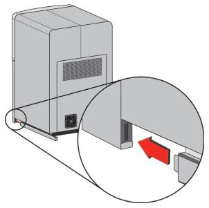
Insert tab in slot and push cover toward front of system
