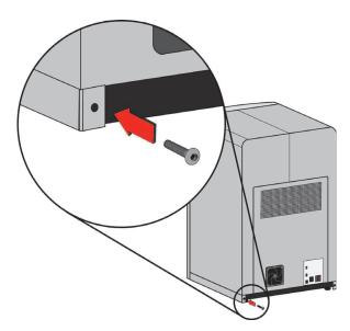
Attach screw at back of system
