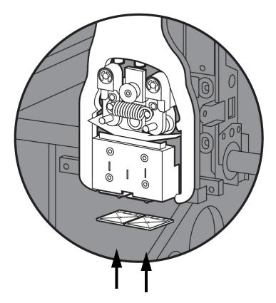
Figure 5-12: Tip shield placement
