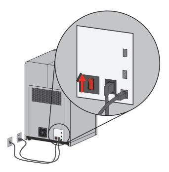
2. Turn the power switch to the on (I) position. See Figure 3-8. After the switch is pushed, the system boots up in three to seven minutes.
