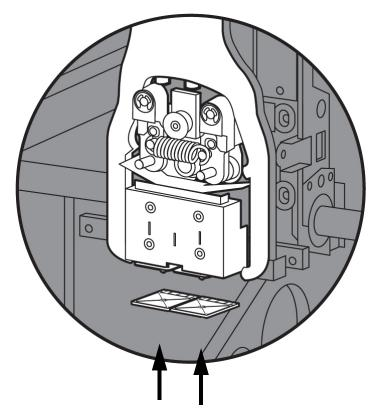
Figure 5-20: Tip shield placement
