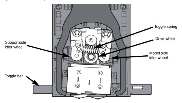
Figure 6-6: Toggle bar in neutral position
