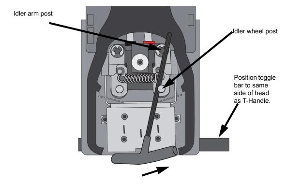
iii. Move idler wheel assembly by pushing with  $\frac{7}{64}$ " T-Handle Allen wrench against spring tension. Insert a  $\frac{1}{8}$ " T-handled Allen wrench (from startup kit) into the fixture hole. See Figure 6-8.
