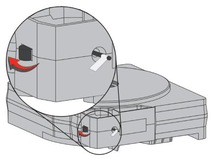
4. Pull material out of cartridge to expose about 12 inches of material. You should easily be able to pull out the material.
