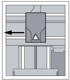
3. Remove the tip wipe assembly by lifting the assembly up and out of the machine. Discard the old tip wipe assembly, see Figure 5-5.
