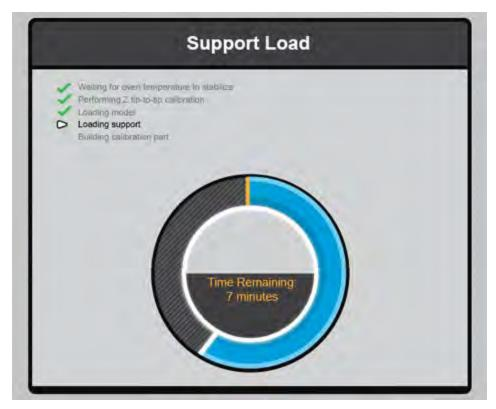
B. In addition to the screen updating, the Information Bar and the Build State button will update to indicate when the printer is building the calibration part.
