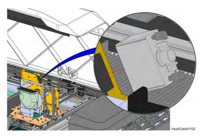
6. Using a  $\frac{9}{64}$ " allen wrench, completely loosen the head mounting screws (2). See Figure 3-18.
