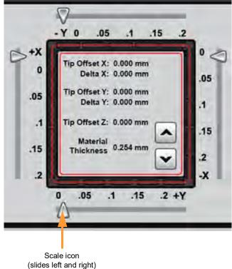
• If the support toolpath is not centered at 2 (0.05 mm) or less (as in Figure 5-10 and Figure 5-12) an offset adjustment is needed. The following figure shows a +X adjustment of 4 or 0.004 in. (0.1 mm). The +X scale icon has been moved downward to the 4 (0.1) and the Delta X value reflects this adjustment (0.0040 in./0.100 mm).
