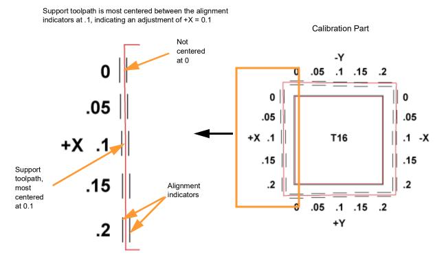
C. Within the Adjust XYZ Calibration page, slide the scale icons on the screen to match where the support toolpath is most centered between the alignment indicators. The Delta X and Delta Y fields will reflect adjustments made.
