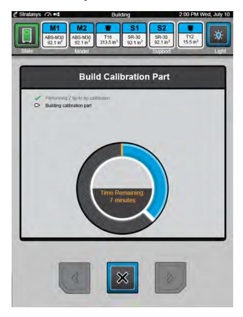
B. Once the calibration part is complete you will be prompted to remove the part from the printer. Remove the build sheet from the platen and allow it to cool and then press the **Next** button to proceed with the wizard.
