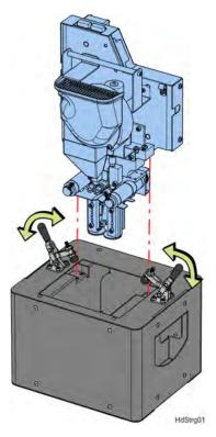
11. Move the head and docking container to a secure storage location.
