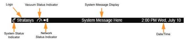
The System Status Indicator (nautilus shell icon) acts as the printer's "heartbeat"; when the printer is functioning correctly, the indicator will slowly flash on and off.
