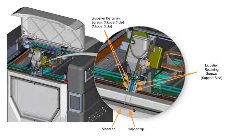
5. Install a new tip into the head (see "Tip Compatibility & Selection" on page 41 for tip/material compatibility information) and then tighten the two (2) liquefier retaining screws using the 9/64 Hex Ball End Driver tip change tool.
