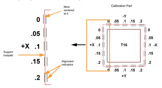
Figure 6-13: Calibration Part - Adjustment Needed (Metric units)
