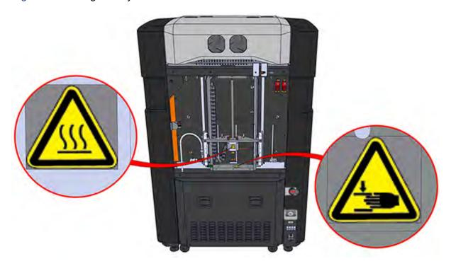
Figure 1-4: Air system safety label locations
