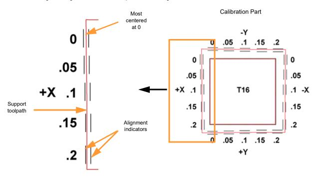
Figure 5-12: Calibration Part - Adjustment Needed (Metric units)
