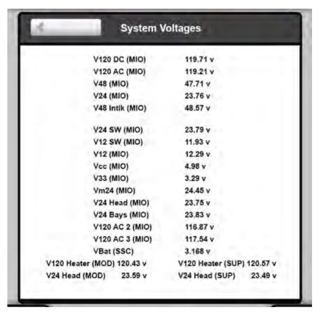
If one or more voltages are out of specification it will be indicated within the Out of Spec Voltages row using red text. The name of the component that is out of spec will be displayed within the row along with a value of 0, indicating that voltage information for the corresponding component is not available.
