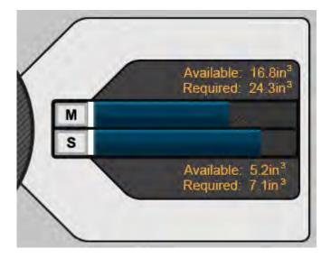
When the printer is building an additional progress bar is displayed for both the model and support fields. This light blue bar indicates build progress and reflects the amount of material used so far during the build.
