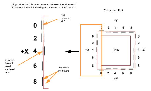
Figure 6-12: Calibration Part - No Adjustment Needed (Metric units)
