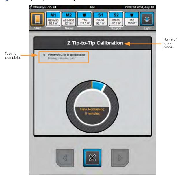
A. In addition to the screen updating, the Information Bar and the Build State button will update to indicate when the printer is building the calibration part.
