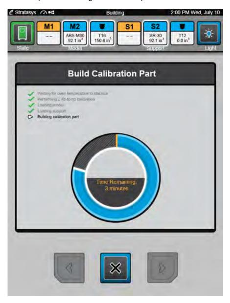
C. Once the calibration part is complete you will be prompted to remove the part from the printer. Remove the completed part and then press the Next button to proceed with the wizard.
