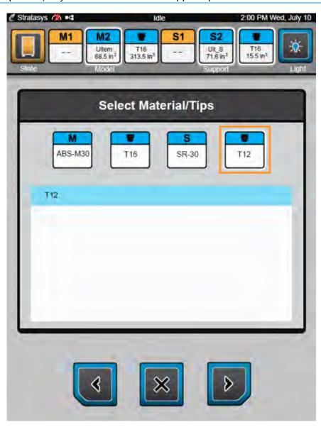
6. Verify that the material and tip selections displayed are correct. If you need to change your material and/or support tip selections, press the **Previous** button and make changes as needed. Ensure that a part is not on the platen and then press the **Next** button to proceed with the wizard.
