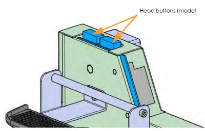
Pressing the **Enable Head Button** button within the Tip Maintenance page makes the corresponding tip's head button active. After pressing this button the tip will begin to heat to a predetermined set point temperature. Once the tip reaches temperature, open the top cover and begin using the tip's head button.
