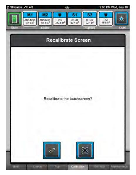
4. A dialog is displayed with instructions for recalibrating the touchscreen. Using a stylus, touch the screen in the center of the calibration point displayed. Repeat this process for the remaining calibration points (1 point for each of the 4 corners of the screen).
