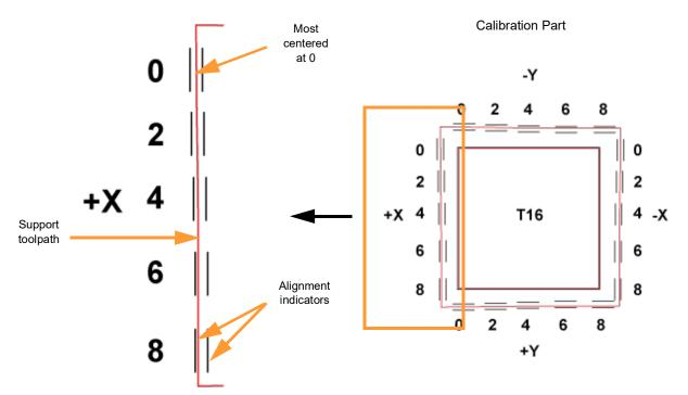
Figure 5-10: Calibration Part - Adjustment Needed (English units)
