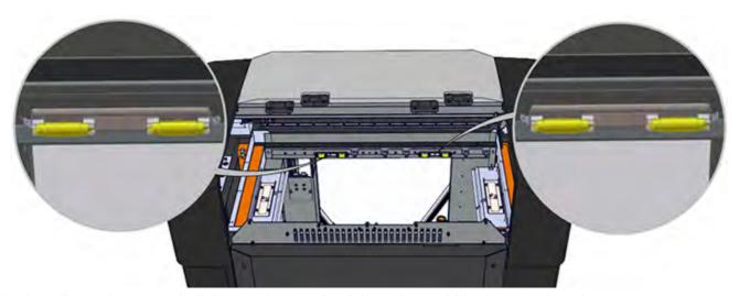
4. Install a replacement bulb by gently pressing it into place within the securing clamps.
