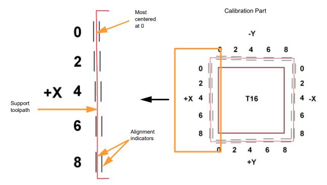
Figure 6-11: Calibration Part - Adjustment Needed (English units)
