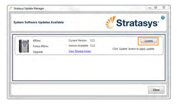
9. The application will begin sending software to the printer. Once the software download is complete, you will need to reboot the printer to complete the update.
