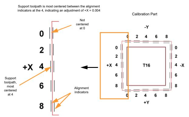
Figure 5-11: Calibration Part - No Adjustment Needed (Metric units)
