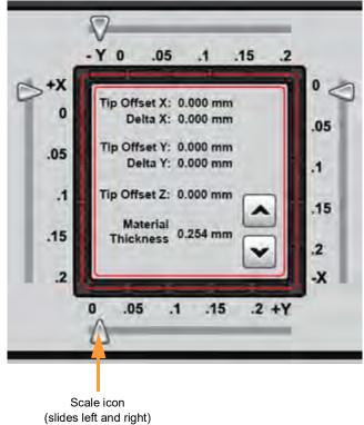
• If the support toolpath is not centered at 2 (0.05mm) or less (as in Figure 6-11 and Figure 6-13) an offset adjustment is needed. The following figure shows a +X adjustment of 4 or 0.004 in. (0.1 mm). The +X scale icon has been moved downward to the 4 (0.1) and the Delta X value reflects this adjustment (0.0040 in./0.100mm).
