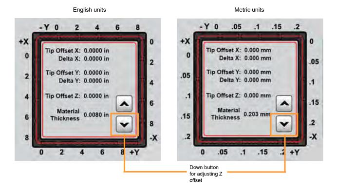
Use the Up button to enter the value obtained in step C if this value is greater than the tip's slice height. For example, if you measured an average of 0.012 in.
