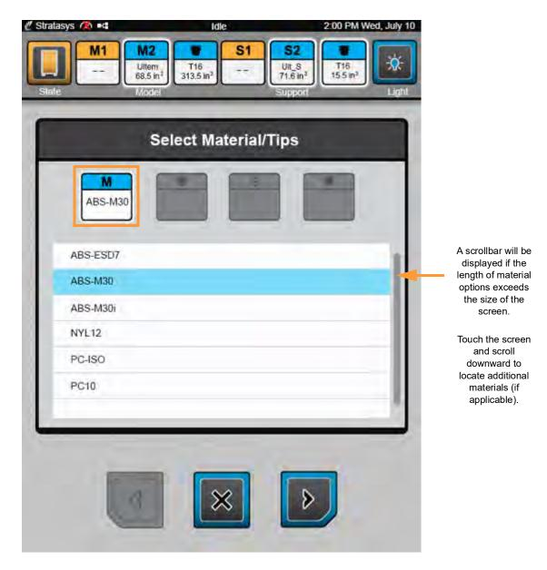
From the list of tip options displayed, select the model tip you'd like to switch to (T16 (new) in this case). The newly selected model tip will be indicated. Press the Next button to proceed with the wizard.
