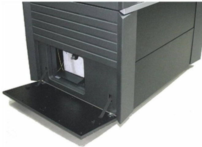
Figure 6-129 Accessing the waste container
