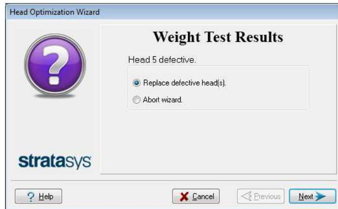
Figure 6-66 Defective print heads found
