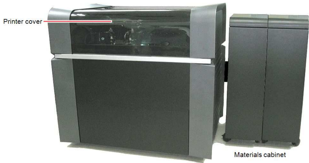
Figure 6-1 The Stratasys J750 3D Printer
