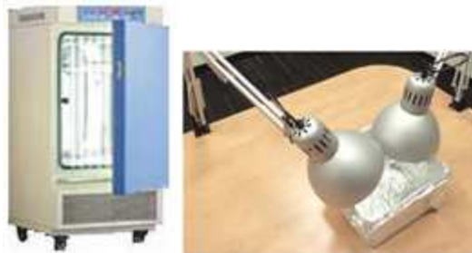
Figure 7-2 Left: Illumination chamber; Right: Desk lamps
