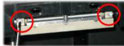
Figure 6-42 Removing the roller waste collector
