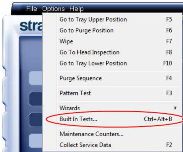
Figure 6-126 Selecting Built-In Tests from the Options menu
