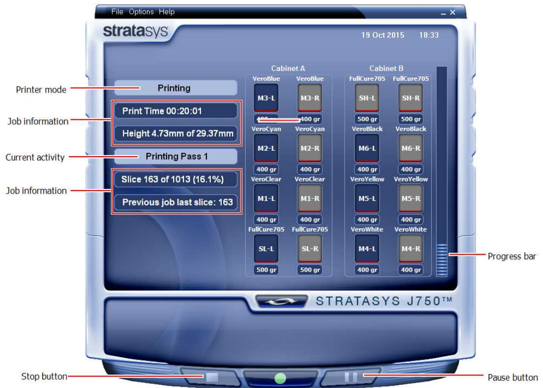
Figure 6-5 Printer interface during printing
