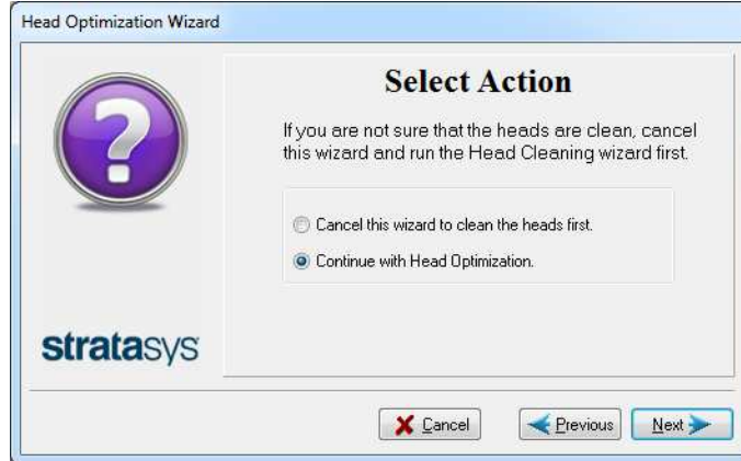
Figure 6-67 Clean print heads screen
