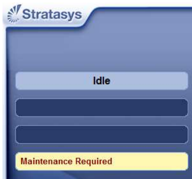
Figure 6-30 Maintenance Required indicator
