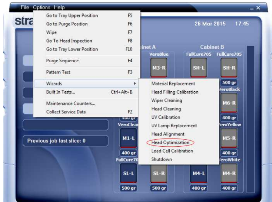
Figure 6-54 Starting the Head Optimization wizard
