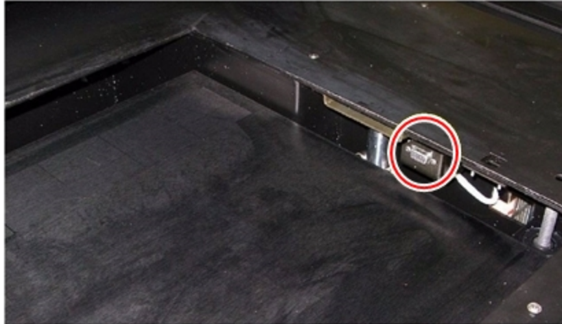
Figure 6-92 UV sensor connector
