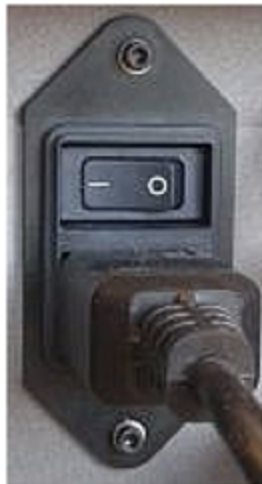
Figure 6-2 Main power switch and cable
