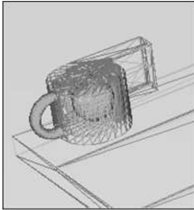
Figure 5-39 Build tray and model displayed in WireFrame view
