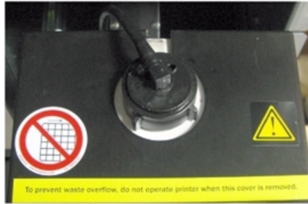
Figure 6-144 Cover installed over the waste container
