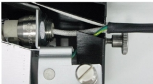
Figure 6-104 Cable position when installing the UV lamp
