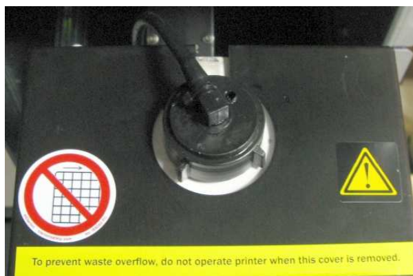
Figure 6-121 Cover installed on the waste container
