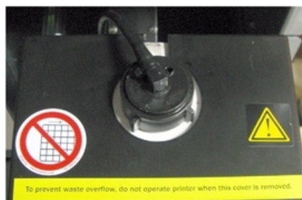
Figure 6-137 Cover installed on the waste container
