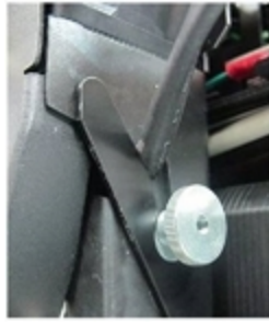
Figure 6-51 UV-lamp cable in place after securing the assembly
