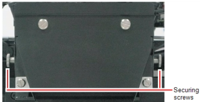
Figure 6-46 UV-lamp-assembly securing screws
