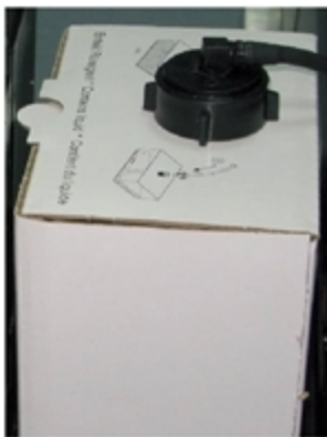
Figure 6-143 Waste container with drain tube attached
