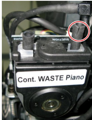
Figure 6-128 Tubes disconnected from the waste pump
