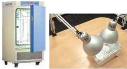
Figure 7-2 Left: Illumination chamber; Right: Desk lamps
