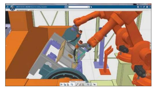
Robot programmers create, program, simulate and validate an entire robot workcell before sending programs and setups to the shop floor.
