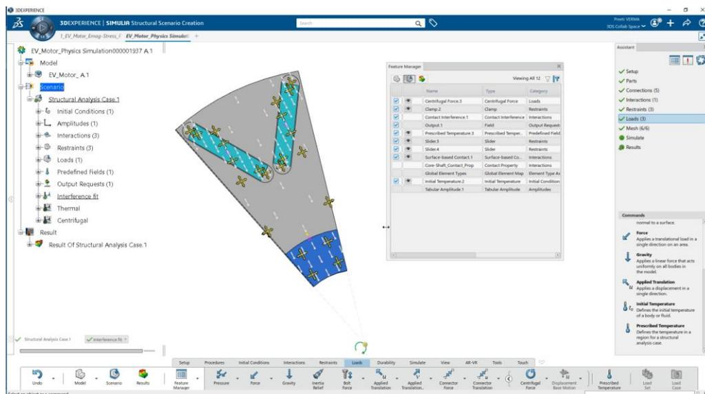
Figure 3.1: Stress Analysis of electric motor section for interference, thermal and centrifugal loading
