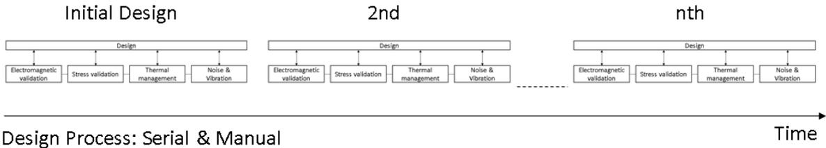
Figure 2.2: Serial and Manual Design Process over multiple design cycles
