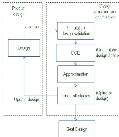
Figure 4.1: Simulation process using a DOE
