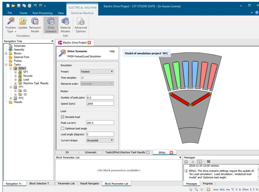
Figure 3.2. Electromagnetic analysis of electric motor in CST Studio Suite
