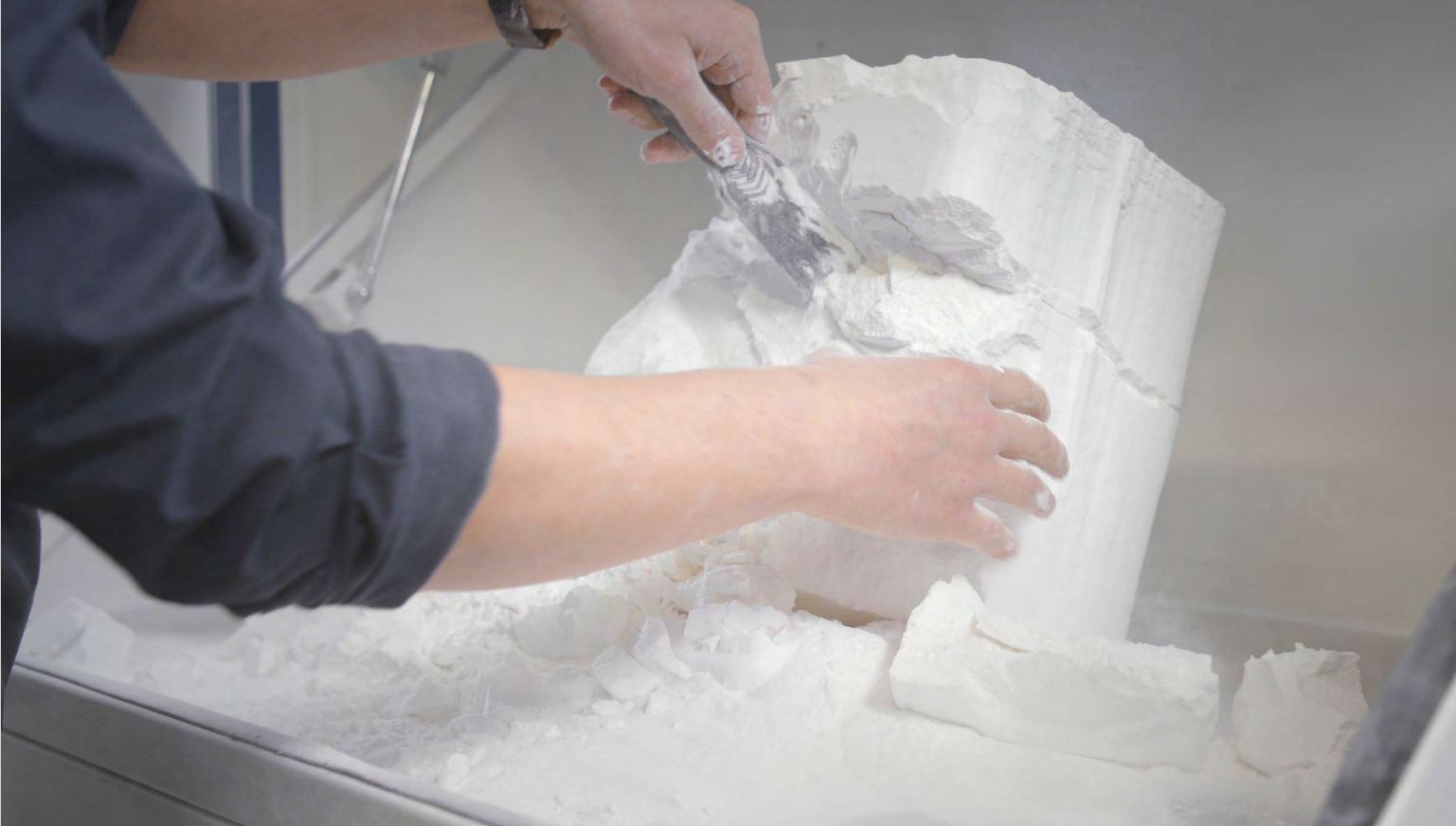
The H350 uses an infrared sensitive HAF™ to fuse particles of polymer powder together in layers to build parts
